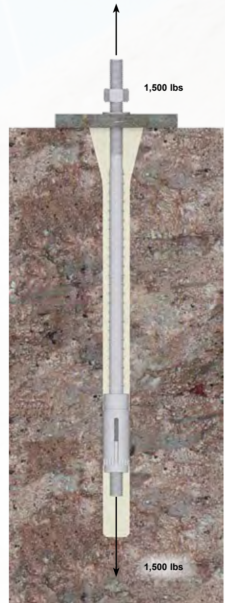
3 External load of 1500 lbs. is applied
