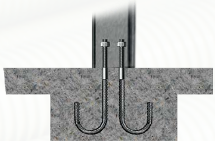
Concrete Column Anchor
