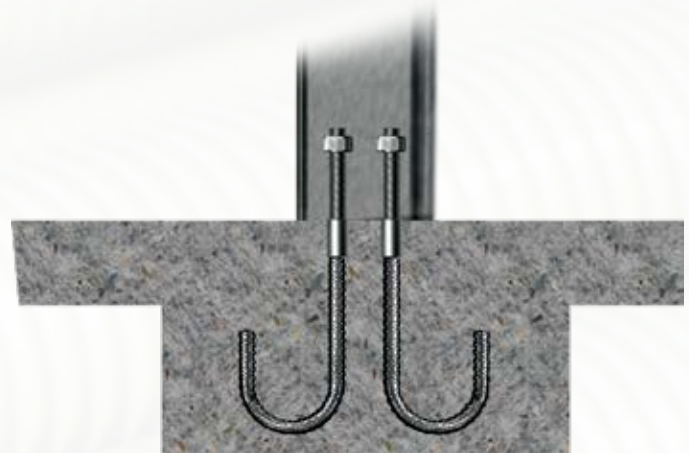
Concrete Column Anchor
