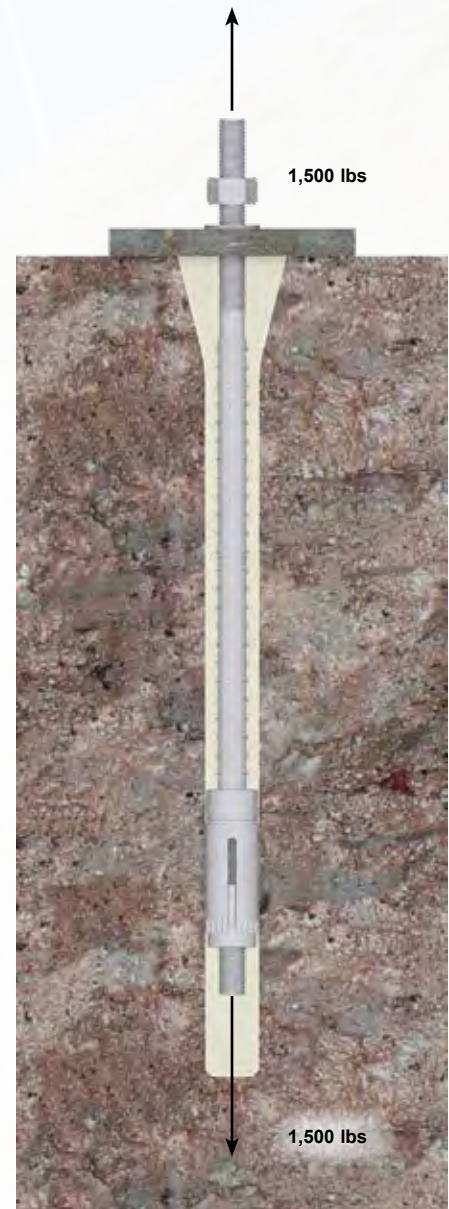
3 External load of 1500 lbs. is applied
