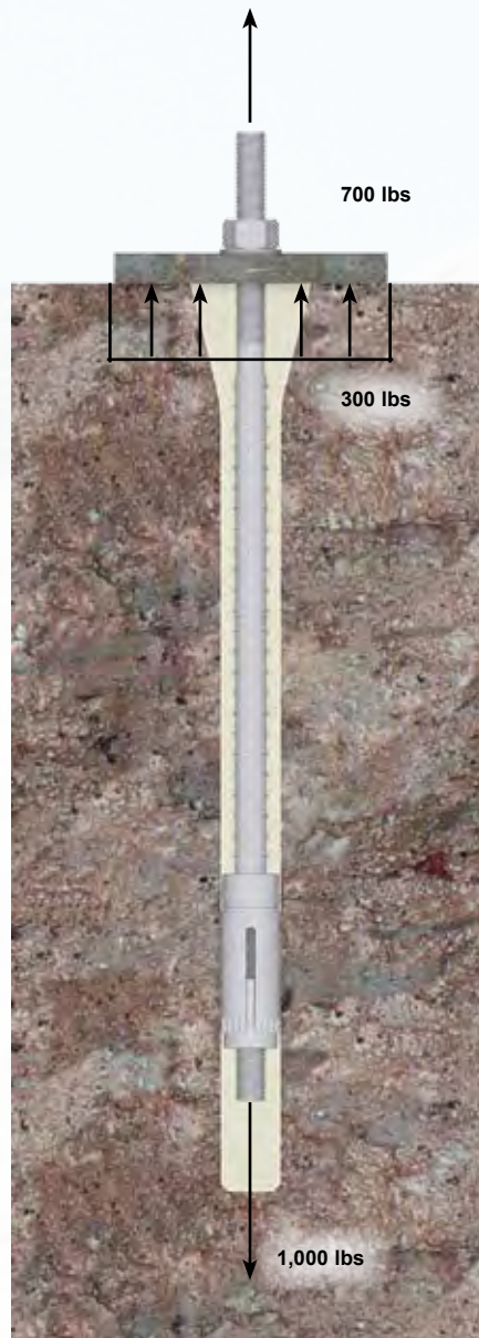
2 External load of 700 lbs. is applied to the anchor
